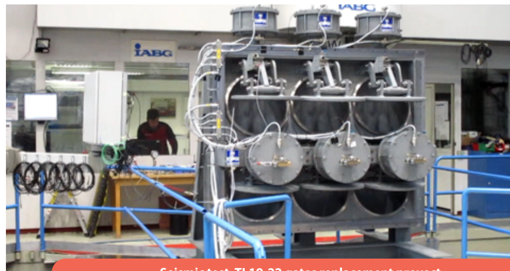
Seismic test, TL19-22 gates replacement project
